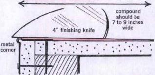
Be sure the metal corner is attached firmly. Take your 4" finishing knife and spread the G-P Ready-Mix 3" to 4" wide from the nose of the bead, covering the metal edges. When completely dry, sand lightly and apply second coat, feathering edges 2" to 3" beyond the first coat. A third coat may be needed depending on your coverage. Feather the edges of each coat 2" or 3" beyond the preceding coat.
