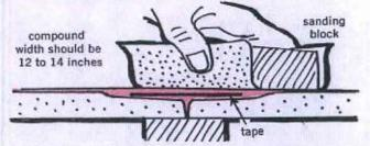
When thoroughly dry, at least 24 hours, apply a fill coat extending a few inches beyond the edge of the tape and feather the edges of the compound. When the first finishing coat is thoroughly dry, use your 10" joint finishing knife and apply a second coat and feather the edges about  $1\frac{1}{2}$ " beyond the first coat. When this coat is dry, sand lightly to a smooth even surface. Wipe off the dust in preparation for the final decoration. Total width should be 12 to 14 inches.
