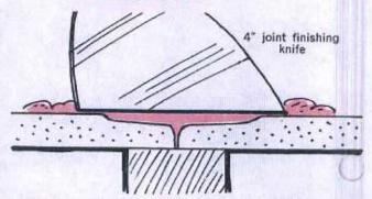
Take your 4" joint finishing knife and apply the Ready-Mix Joint Compound fully and evenly into the slight recess created by the adjoining tapered edges of the board.
