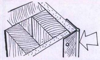
To protect corners from edge damage, install metal cornerbead after you have installed the wallboard. Nail the metal cornerbead every 5" through gypsumboard into wood framing.
