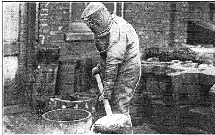
MASK OF WIRE CLOTH WITH ADJUSTABLE CAP AND APRON OVER NECK AND CHEST FOR PROTECTION IN BABBITTING AND SIMILAR OPERATIONS
