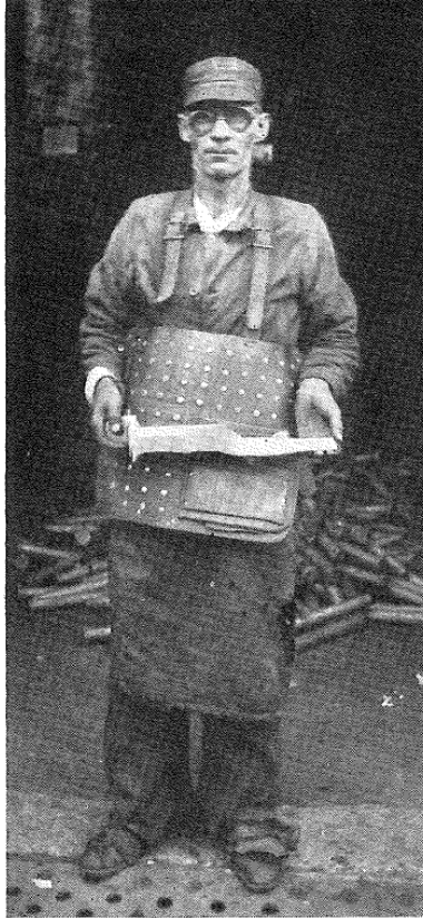
F IGURE 1: Steel-bradded leather aprons are worn by casting grinders at the American Steel Foundries to protect the abdomen from vibrations
